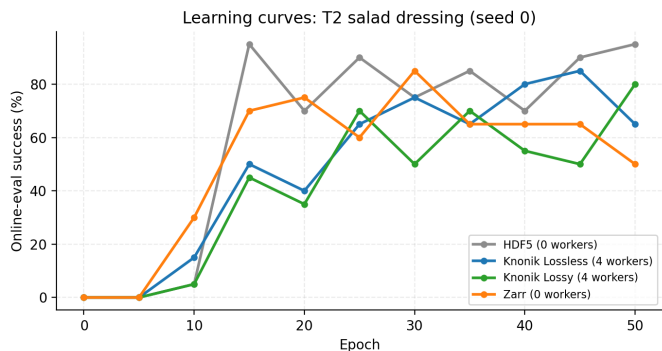
Fig. 18. Online-eval success curves for T2 salad dressing (seed 0) across all four formats. Zarr and lossless reach the same peak (85%); HDF5 peaks higher (95%) on this seed; both Knonik modes converge earlier than the single-process loaders.
