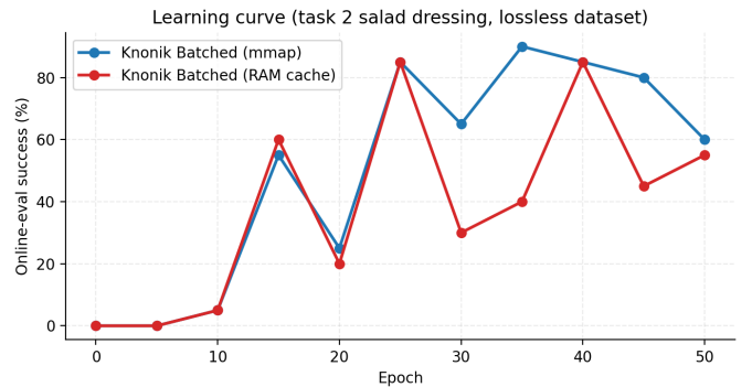
Fig. 14. Online-eval success curve (20 rollouts at training time) on T2 salad dressing under each cache mode. Both modes follow the same qualitative trajectory; the mmap run reaches a slightly higher per-epoch peak (90% vs. 85%) and a higher final-epoch success (60% vs. 55%).
